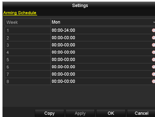
Figure 8. 16 Set Arming Schedule of Alarm Output
