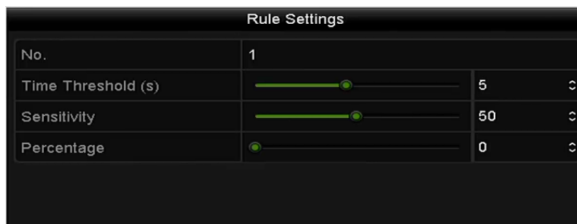
Figure 9. 8 Set Intrusion Crossing Detection Rules
