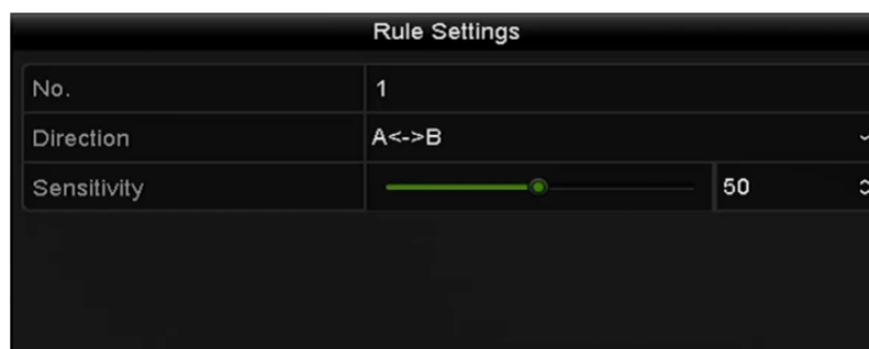
Figure 9. 6 Set Line Crossing Detection Rules
