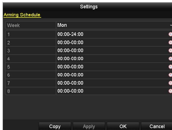
Figure 8-17 Set Arming Schedule of Alarm Output
