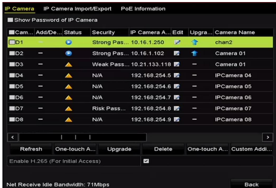
Figure 2-22 IP Camera Management Interface
