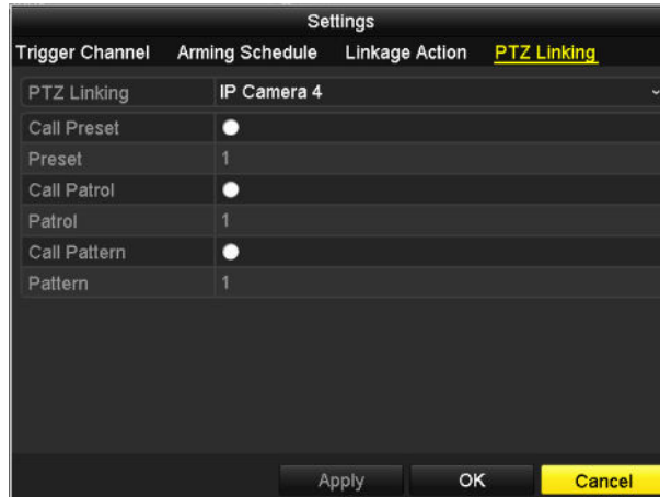
Figure 8-7 Set PTZ Linking of Alarm Input
