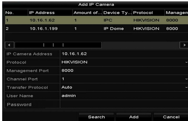
Figure 2-25 Quick Adding IP Camera Interface
