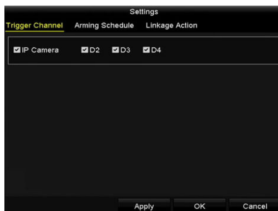
Figure 5-18 Set Trigger Camera of VCA Alarm
